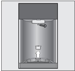
■ Remove the screw from the rear casing, then lift the tab on the drip tray up and off.
